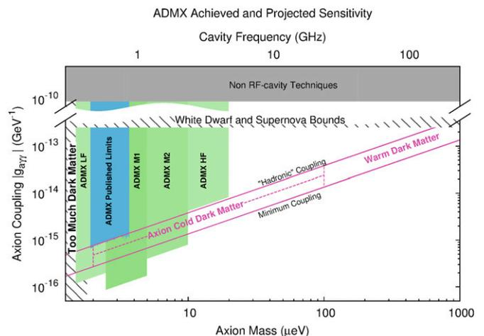
Fig. 4. Sensitivity reach of ADMX over the next several years. This experiment will have the sensitivity to detect the dark-matter QCD axion or reject the hypothesis at high confidence.
