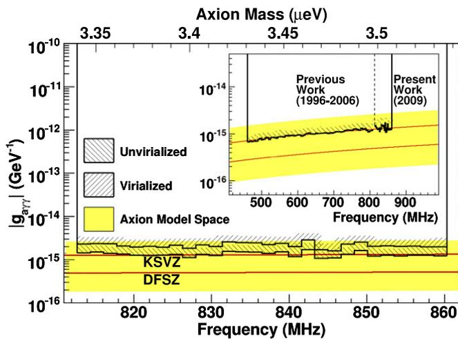
Fig. 3. Recent results from ADMX SQUID operation without a dilution refrigerator. The ADMX experiment is sensitive to plausible axion couplings in the dark-matter axion window.
